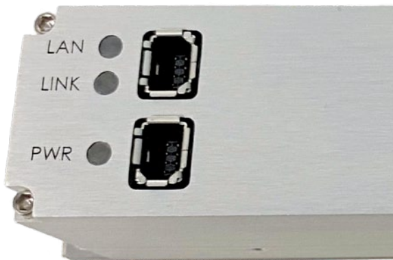
FIGURE 2-7: POWER & ETHERNET CONNECTIONS - EPX
